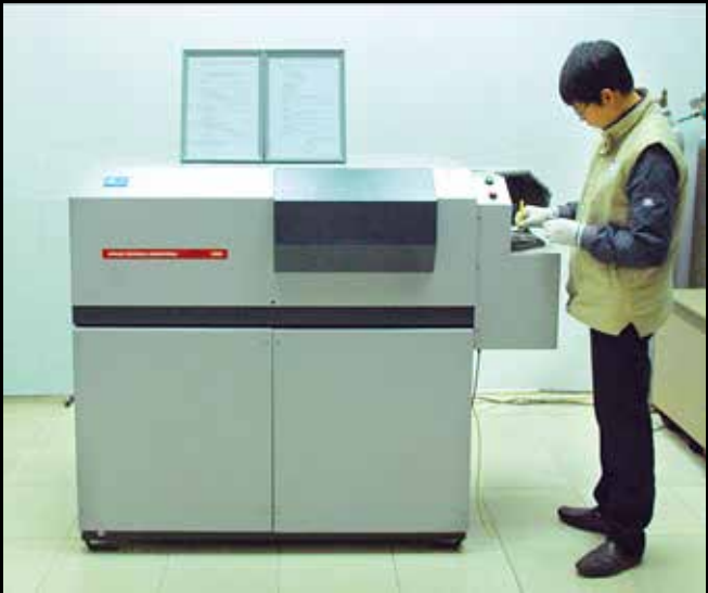
ARG optical emission spectrometer Metals Analyzer of 24 elements( Switzerland)
