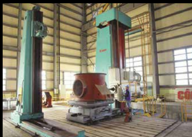
Boring machine W250 Machining capacity: X/Y/Z 7000 2000 4000mm
