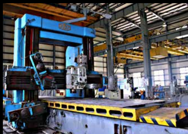
Bed sharpening machine HC13T Machining capacity: X/Y/Z 8000 1800 1500mm
