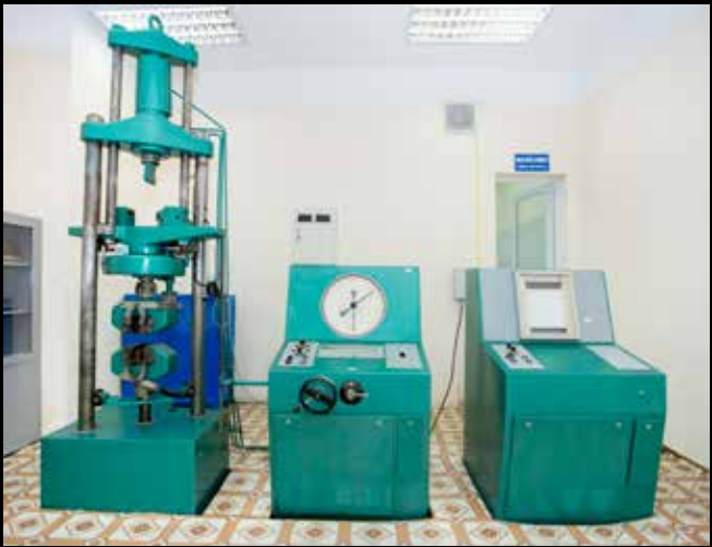
300 KN Tensile-Strength-Stress-Strain testers
